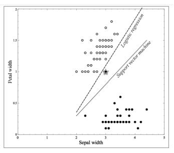
**Figure 10.** Using logistic regression and SVM to separate binary classes [34, p.89]. For classification in a scenario containing more classes, the multinomial logistic regression [25].
