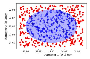
**Figure 16.** Five hundred test data were used to make the predictions. Points blue marked with "+", inside the circle, are within the values specified by the customer.
