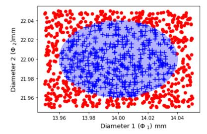
**Figure 15.** One thousand dice are used for training. Points blue marked with "+", inside the circle are within the values specified by the customer.
