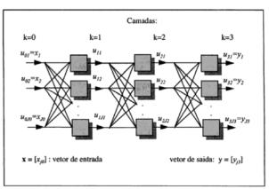
Figure 12. Four-layer neural network (multilayer perceptron) [36, p. 40].
