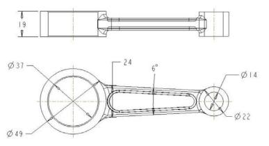
Figure 1. Structure of a connecting rod with its specified dimensions [6].
