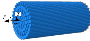
Fig. 5. Boundary conditions of tension and torsion combined
