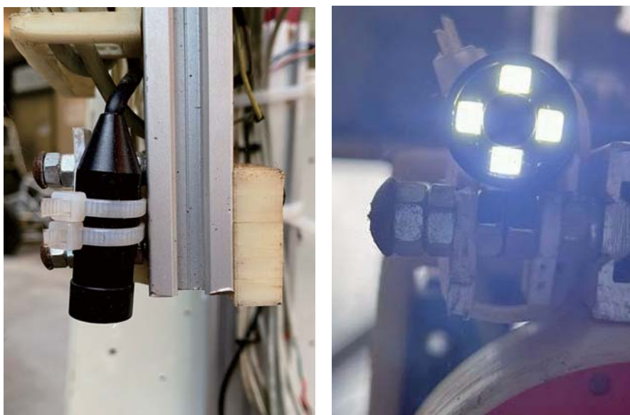
Figure 7. Borescope camera fixed mounted on the tip of the Z-axis arm.
